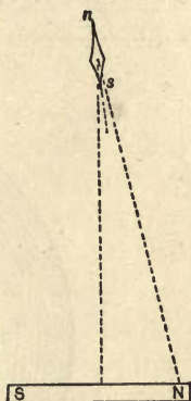
DEFLEXION OF NEEDLE CAUSED BY BAR MAGNET BROADSIDE-ON.
